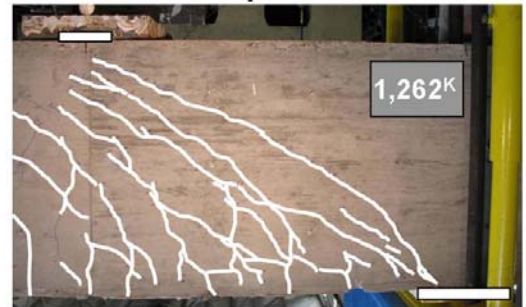
Figure 4-14: Comparison of cracking patterns at maximum applied load
