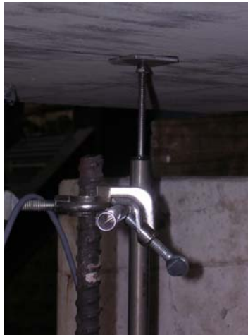
Figure 3-21: 6-inch linear potentiometer
