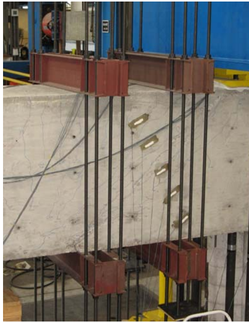
Figure 3-7: Strengthening of a beam after strut failure: external PT clamp
